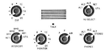
The knob labeled MONITOR in the above picture controls the speakers above the DJ's head. The monitor dial does not affect the meters, or what the listeners hear, just the volume you hear in the studio.
